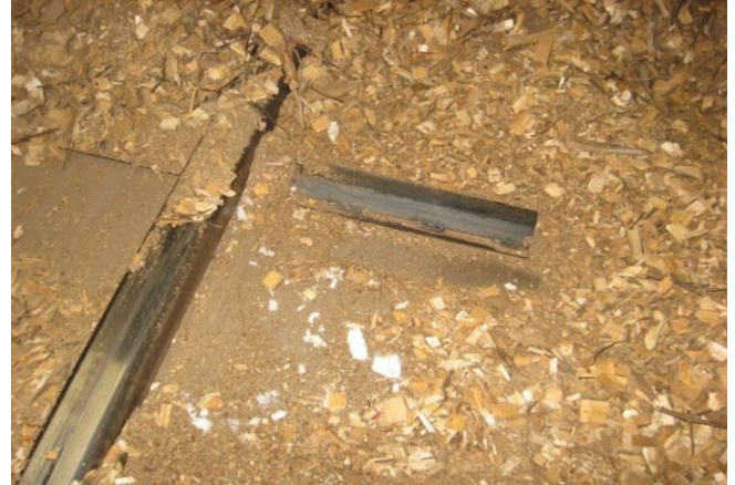
Figure 5: A walking floor consists of horizontal bar dischargers moving back and forth. Photo: Jyrki Raitila, VTT.
