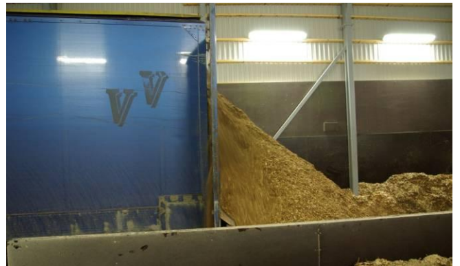
Figure 6: Chips being delivered; the truck has bar conveyors for unloading. Photo: Jyrki Raitila, VTT.
