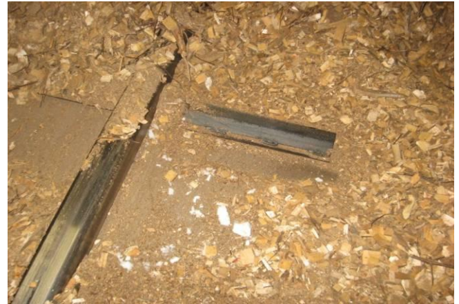
Figure 6: A walking floor consists of horizontal bar dischargers moving back and forth. Photo: Jyrki Raitila, VTT.
