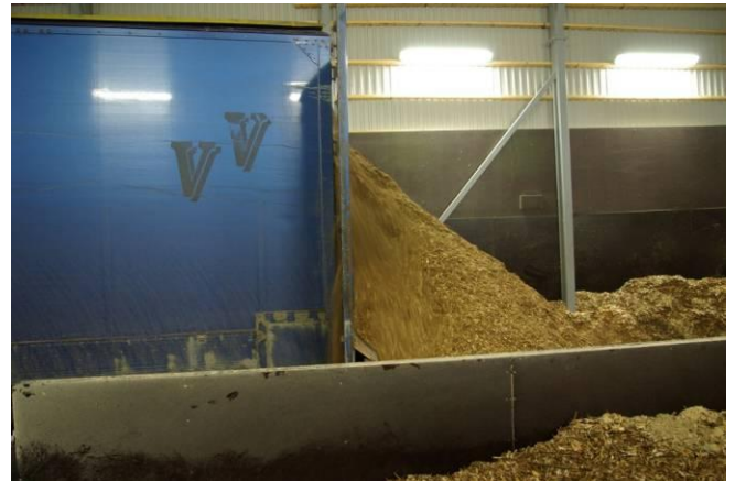
Figure 5: Chips being delivered; the truck has bar conveyors for unloading. Photo: Jyrki Raitila, VTT.
