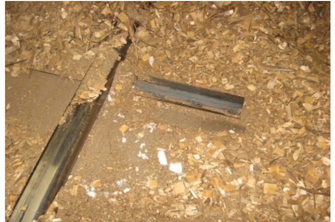
Figure 4: A walking floor consists of horizontal bar dischargers moving back and forth. Photo: Jyrki Raitila, VTT.
