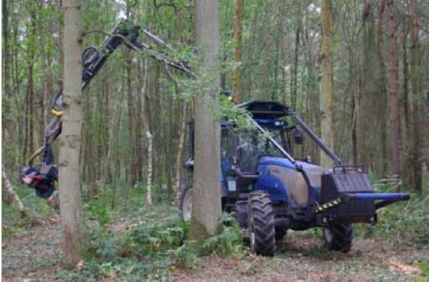
Valtra tractor (second hand) with 8 metre reach Botex arm and Keto processing head. Note:
